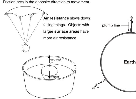
Objects **appear to weigh less** in water because of **upthrust**.
